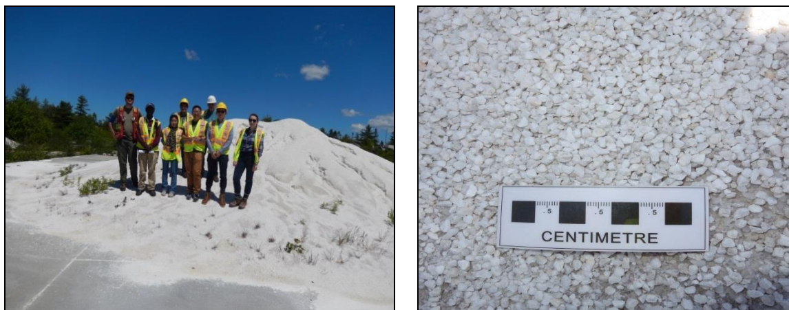
Figure 2: A group photo standing on one of the white rock (kaolinite and quartz) pile (a); and a close-up photo of the quartz crystals with interstitial kaolinite (b).
