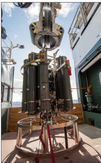
Figure 4: The CTD (Conductivity-Temperature-Depth) device.
