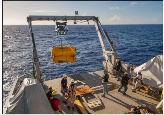
Figure 7: Deploying the AUV Sentry (WHOI).
