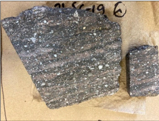
Figure 8: Close-up of a basal vitrophyre of intracaldera Stone Cabin tuff. The tuff includes quartz, feldspar, and biotite.
